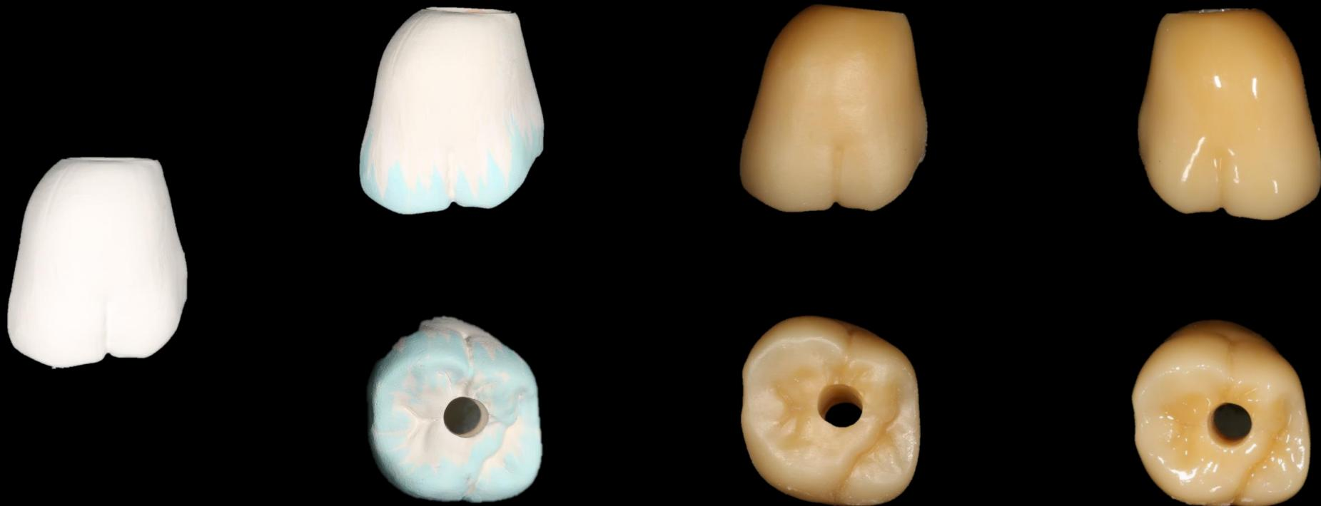
Milling / Coloring / Sintering / Glazing
